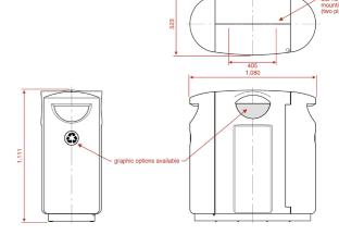
Proposed: Cast Ductile Iron litter bin with 3 compartments; litter and recycling.
