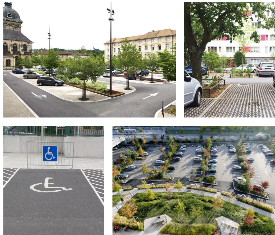
TL: Successful town centre car parking integrated with a landscaping scheme TR: The use of multiple surface materials to add texture and visual interest. BL: Disabled parking bay and sign, Ireland BR: Efficient car park layout with clear pedestrian routes and furniture.
