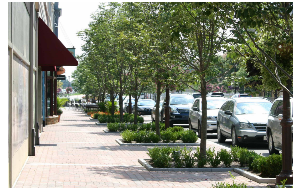
Proposed: widen pavements and introduce planting to limit vehicles encroaching the pavements to park.
