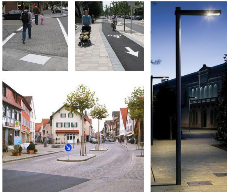
TL: Use of differentiated paving to strengthen the visibility of the crossing
