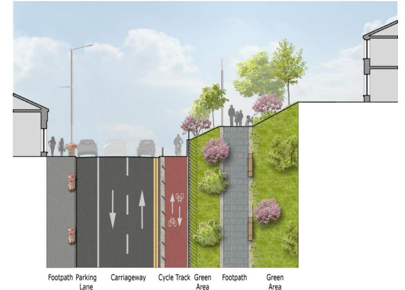
*Proposed: redesign Dublin Road section with the introduction of a cycle lane and of a footpath protected from adjacent traffic.*
