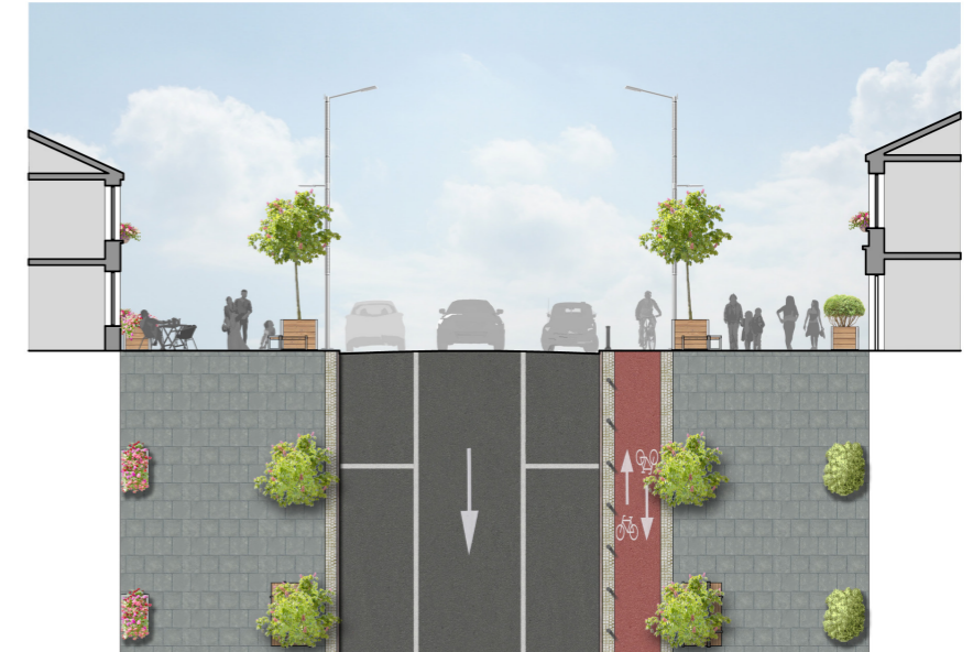
Proposed: New Market Street section with widened pavements, added street furniture and planting, parallel parking and cycle lane.
