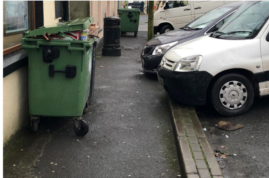
Ballinagh - existing: uneven paving cluttered with furniture and current design enables parked cars to overlap the kerb.
