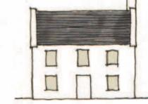
A 30 degree roof pitch is recommended
