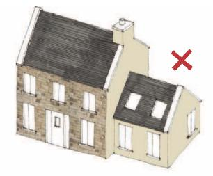
When using stone as an external material create '3d' elements (by using 3 to 4 faces of part or all of the building) rather than cladding one face.
