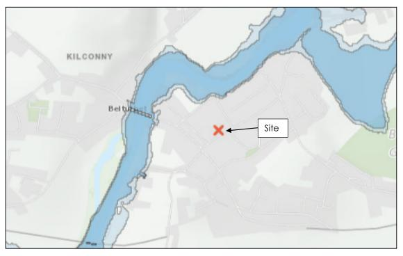
Fig 3.3 Extract of CFRAM mapping showing extents of Fluvial flooding
