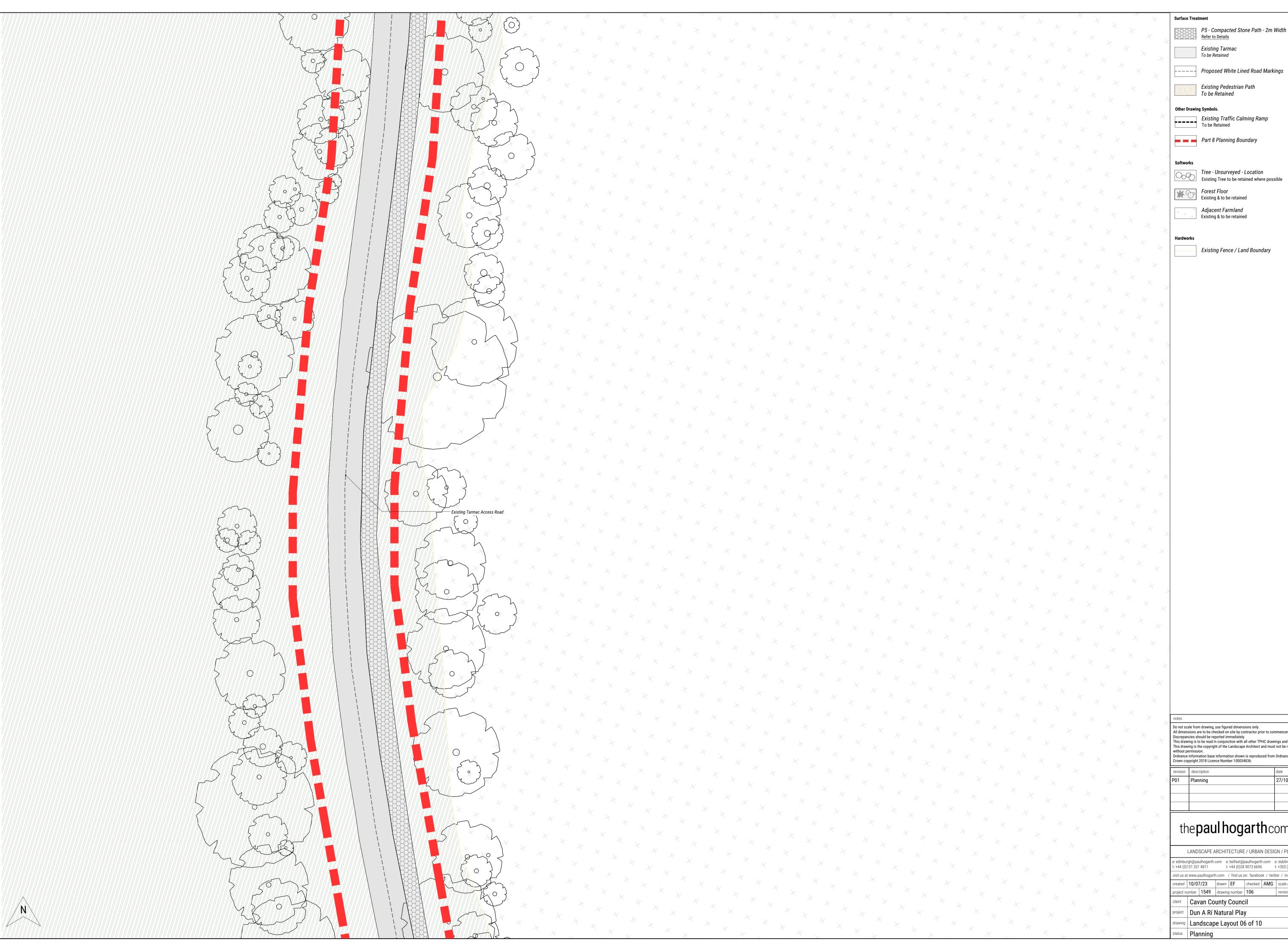
Refer to Details Existing Tarmac To be Retained ---- Proposed White Lined Road Markings Existing Pedestrian Path To be Retained Other Drawing Symbols. Existing Traffic Calming Ramp To be Retained Part 8 Planning Boundary Tree - Unsurveyed - Location Existing Tree to be retained where possible Forest Floor Forest Floor
