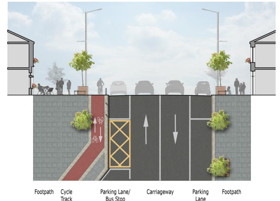
Proposed: a reduction in the total width of the carriageway could allow for a cycle lane and spill out areas for cafés, with seating and improved street furniture.
