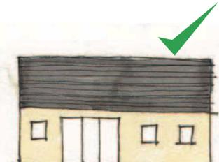
Large void is possible when balanced by small openings
