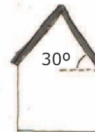
A 30 degree roof pitch is recommended
