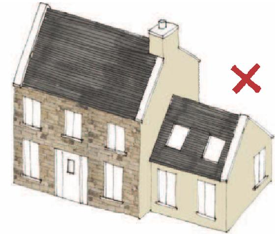
*When using stone as an external material create '3d' elements (by using 3 to 4 faces of part or all of the building) rather than cladding one face.*
