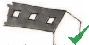
Similar rooflights flush with roof
