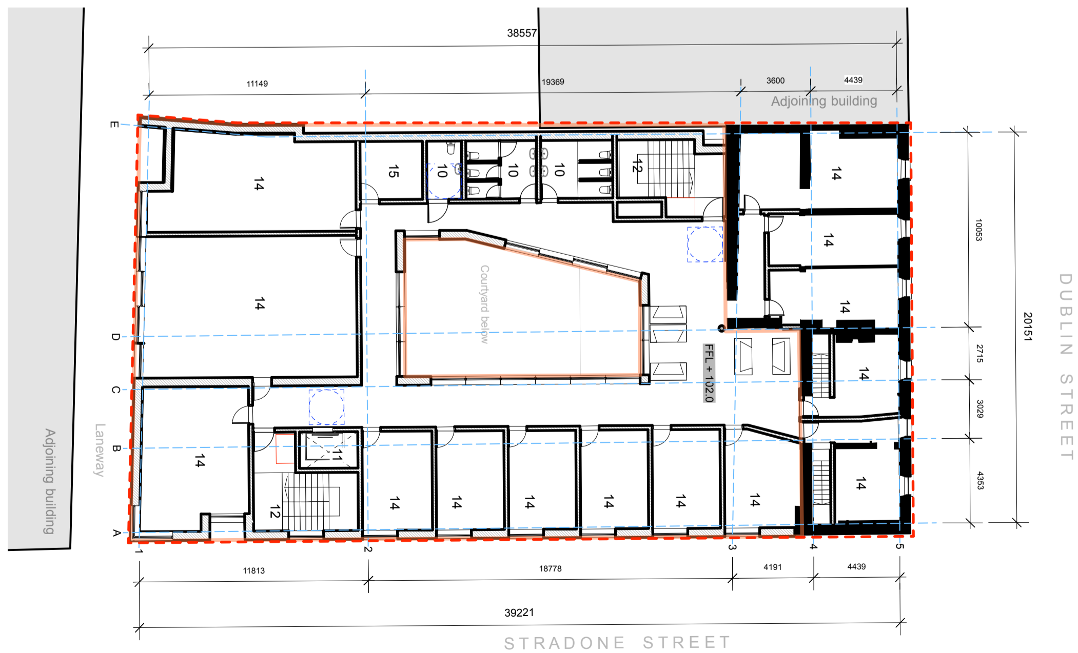
01 Proposed First Floor Plan
