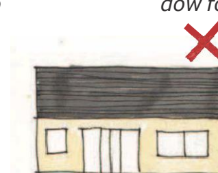
Too many large voids
