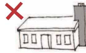
Chimney too large
