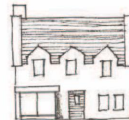
Windows have vertical emphasis
